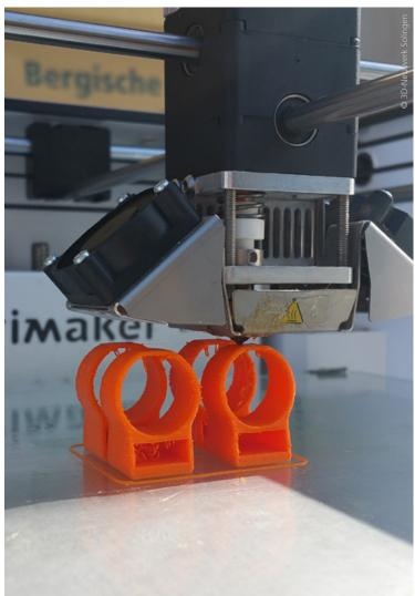
3D print with FDM technology (Fused Deposition Modeling)
