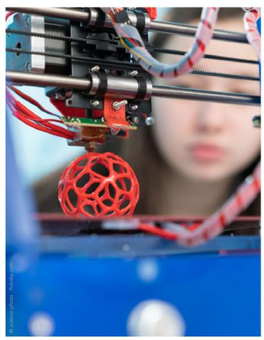
3D print with FDM technology (Fused Deposition Modeling)
