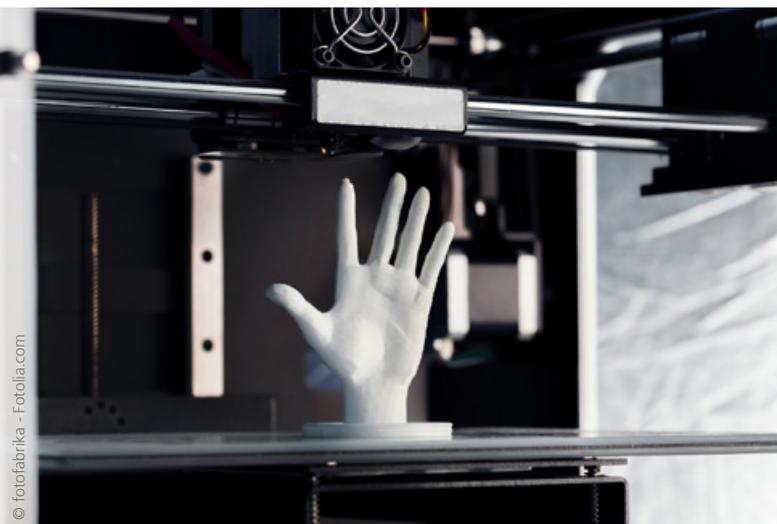
3D printed model of a hand
